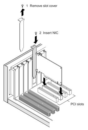
Figure 3 Inserting the NIC
